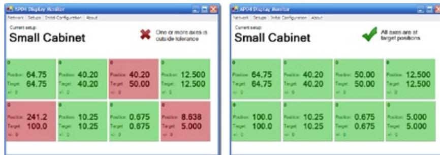
High-end electronic position indicators can be monitored and controlled with a PC or PLC.
